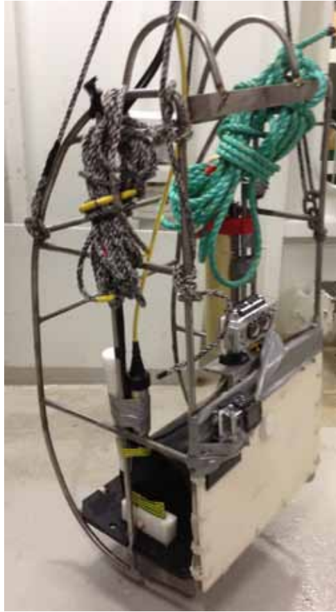
Figure 5.3: Experimental catch monitoring platform, containing, echo sounders (Simrad modified EK 15), camera systems (Go Pro), oxygen logger, STD and tilt logger.
