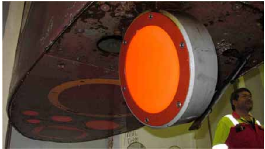
Figure 5.1: The new, narrow beam broadband transducer, experimental installation at the bottom of the drop-keel of G.O. Sars.
