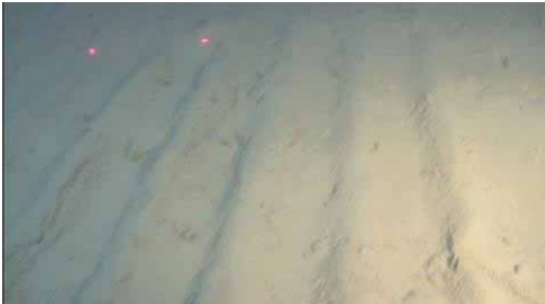
Figure 5.3. Marks created by a sweep chain in soft mud in Varangerfjorden. You can see small heaps of mud spread across the chain tracks. The distance between the red laser lights is 10 cm (from DEGREE 2010).
